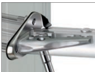
C-sections and F-sections. Lower shroud attached to the spreader bracket.
