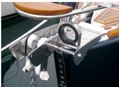
Bow bracket integrated with bow anchor fitting.
