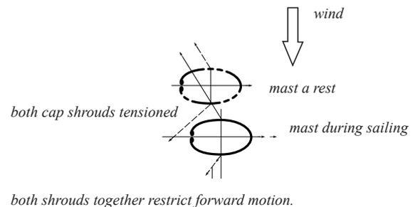
Fig. 1b. Incorrectly tuned cap shrouds
