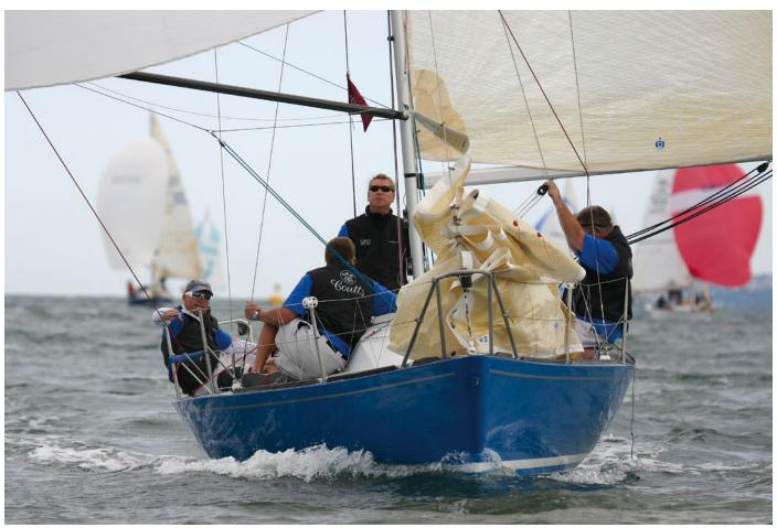
Seldén spinnaker poles are designed to make light work of spinnaker handling. The big advantage of carbon fibre is its low weight. The weight savings enable the crew to handle the spinnaker faster, with less effort.
