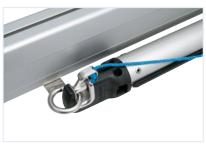
Forward fitting. Can be fitted in the lower end track...
