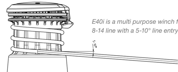
E40i is a multi purpose winch for any 8-14 line with a 5-10° line entry angle.
