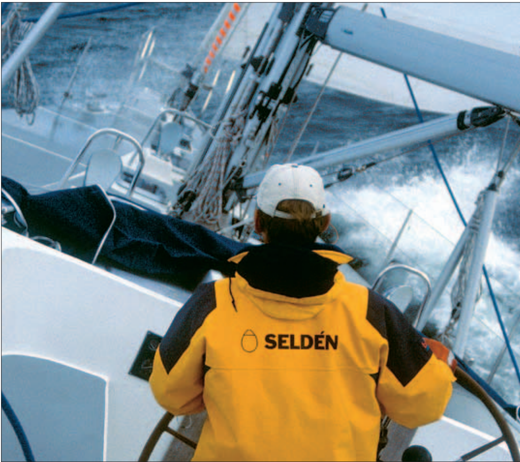
Långedrag 501 equipped with Seldén hydraulic furling mast, hydraulic outhaul and double hydraulic Furlex jib-reefing systems.
