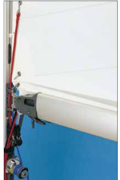
Slab reefing with running S-hooks.
