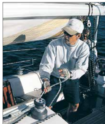
If necessary, apply more main halyard tension.
