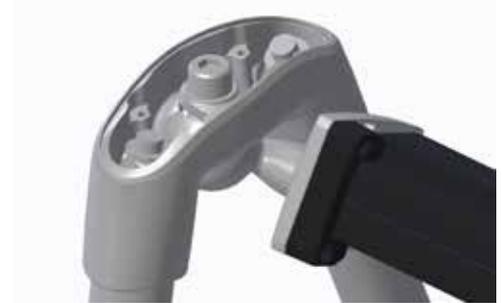
Fit the two lids with M4 screws.
