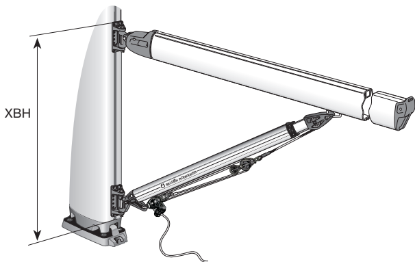
Operation from mast.
