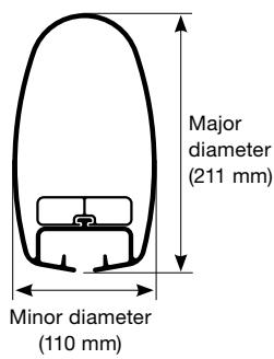
Mast section measurements are given as follows: Major diameter/Minor diameter (i.e. 211/110). This will help identification and the use of correct measurements. The major diameter of the mast can usually be found in the number engraved at the mast heel. For example K23-C211-4475.
