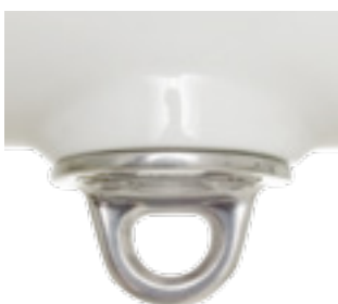
Mainsheet pad eye faired in to underside of the boom.
