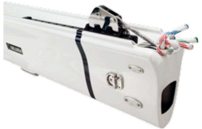
Outboard end showing outhaul track and car, concealed sheaves and pad eye for preventer.
