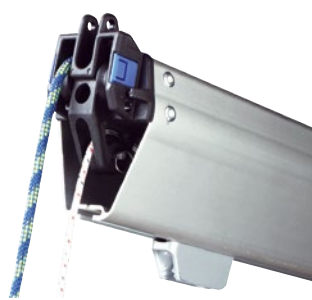
Lead options Additional to the integral gooseneck lock, the inboard boom end fitting offers three sheave lead options for outhaul, reefing lines, flatteners, internal pole retraction systems and anything else you can think of!
