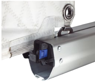
Inboard end The built-in sail feeder (moulded into the fitting) provides a guide for the mainsail clew.
