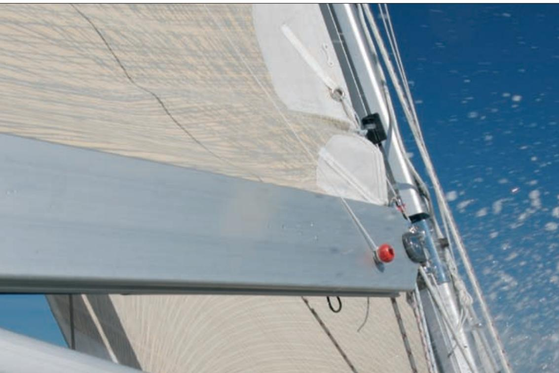
The sail entry gate is designed for use with our MDS cars or with conventional sail slides. When using it with MDS cars, you simply remove the sail entry gate when installing or removing the cars. When using it with conventional slides, use the spring-loaded mid section of the sail entry gate.
