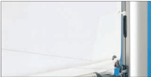
The sail slides are fed in through the spring-loaded gate. When reefing, the sail slides pass through the closed track gate down to the boom, holding the sail in place and facilitating faster and safer reefing. When the spring-loaded section of the track gate is removed, the track gate can just as easily be used with a luff rope.
