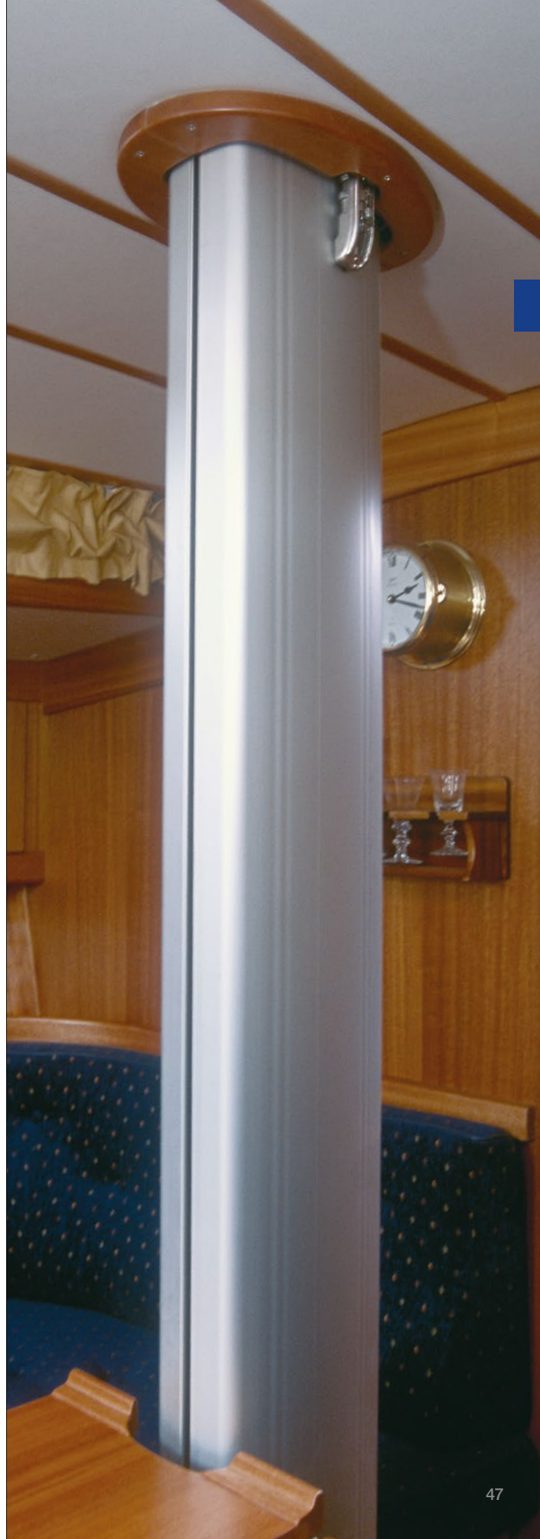
Deck ring with moulded mast coat.
